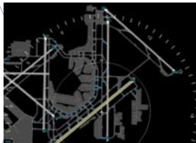
SafeRoute gives a yellow warning to this taxiing aircraft to make the pilot aware that the runway is active.
