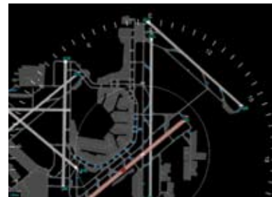
If the pilot ignores the yellow warning and continues onto an active runway, the runway and takeoff aircraft will turn red and an aural alert will be given.
