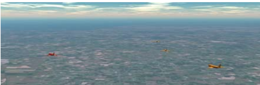
Note the aircraft on the far left. It was given instructions to vector off course because it did not have the proper spacing from the lead aircraft for approach. This procedure wastes time and fuel. With the Merging & Spacing functions, aircraft will be spaced far from the destination aircraft so when they come to the merge point, they will have the proper spacing.
